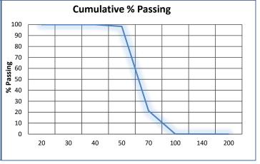
Note: Indicative grading only. Grading analysis may vary from time to time due to changes in raw feed.
